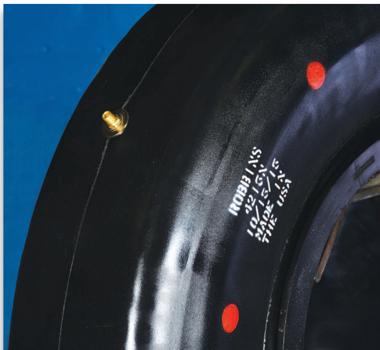
Compression Molding Technology (CMT) from Robbins uses proprietary rubber compounds that are placed into a mold for curing, which eliminates splicing the envelope, increasing production life.
